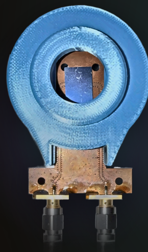
DEDICATED RF ANTENNA & MODULATION COILS
